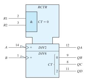
**FIGURE 10.13**Graphic symbol for ripple counter, IC type 7493
