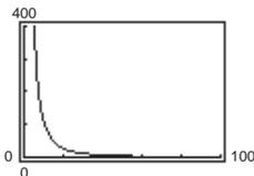
If the diameter is doubled, the resistance is changed by approximately a factor of  $\frac{1}{4}$ . For instance,
