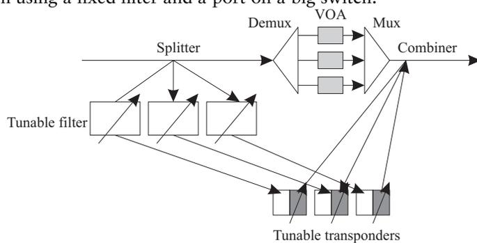
Another plausible OADM architecture is shown above. Here a wavelength blocker device (a demux/mux combination with a per-channel variable optical attenuator) is used to either block the add/drop channels from passing through as well as equalize power levels for the passthrough channels. The loss in the passthrough path is low, but the loss in the add/drop path is high due to the splitters and combiners. However, tunable filters need be provided only for drop channels and not for all channels.
